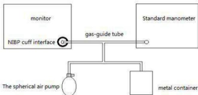
2. The pressure gauge should read zero before inflation. If it is not zero, open the valve of the spherical air pump to make the whole air circuit open to the atmosphere, make the reading of the standard pressure gauge zero, and then close the valve.
