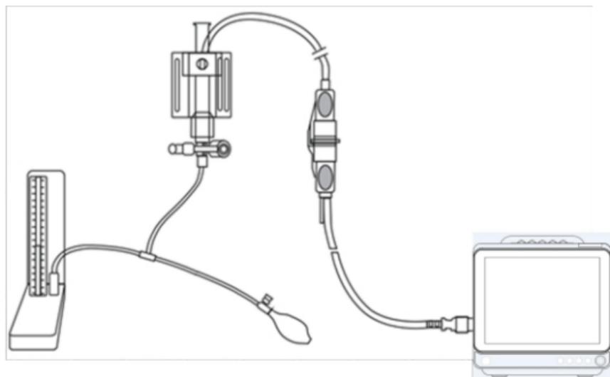
1. Disconnect the pressure transducer from the patient, and connect the three-way stopcock to the sphygmomanometer and inflated balloon with a T-shaped connector, as shown in the following figure;
