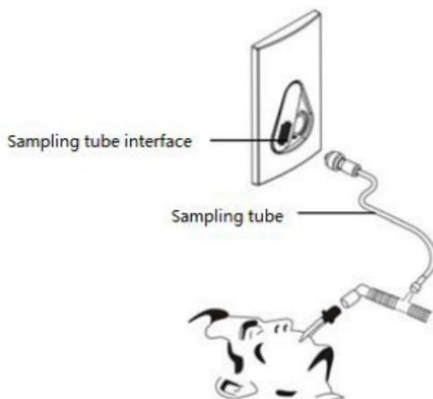
2. The microfluidic CO<sub>2</sub> module defaults to the measurement mode. When the CO<sub>2</sub> module is inserted, the screen displays [CO<sub>2</sub> sensor preheating].
